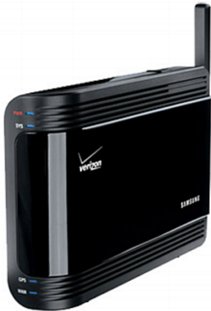
Personal Cell Tower - Femtocell
