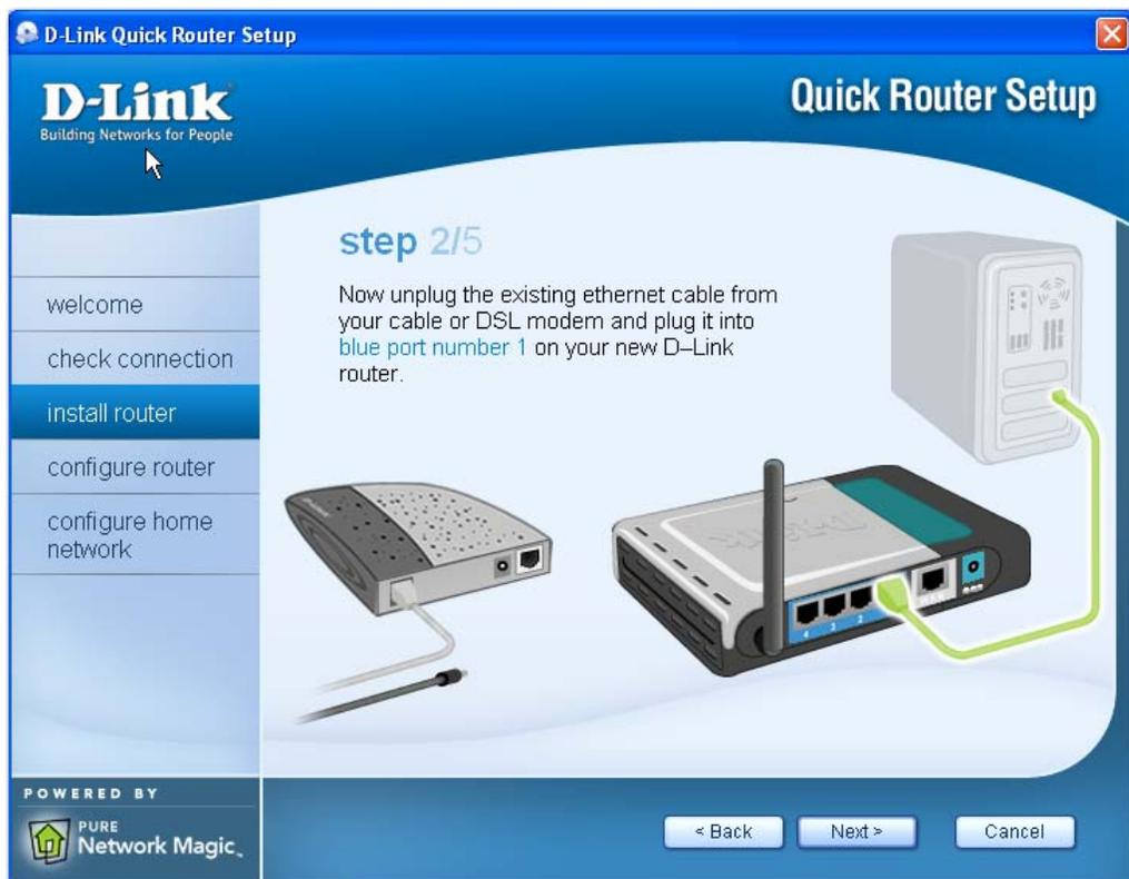
You then are required to plug in the Ethernet cable from the modem to the router and the power cord for the modem.
